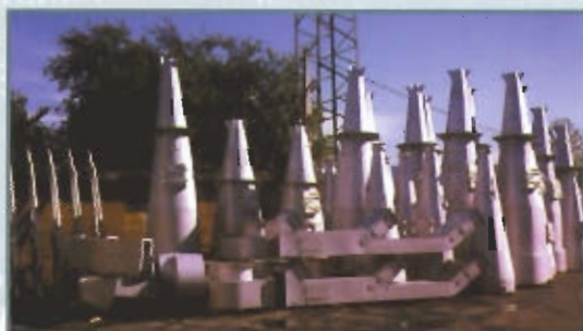
Dedusting cyclones for Dryer UHDE-ALLEMAGNE for IFI-ARKLOW-IRLAND
