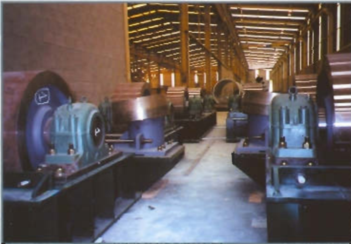
Trunnion rollers in workshop for expedition INSTALLATION ABOCOL-COLOMBIA
