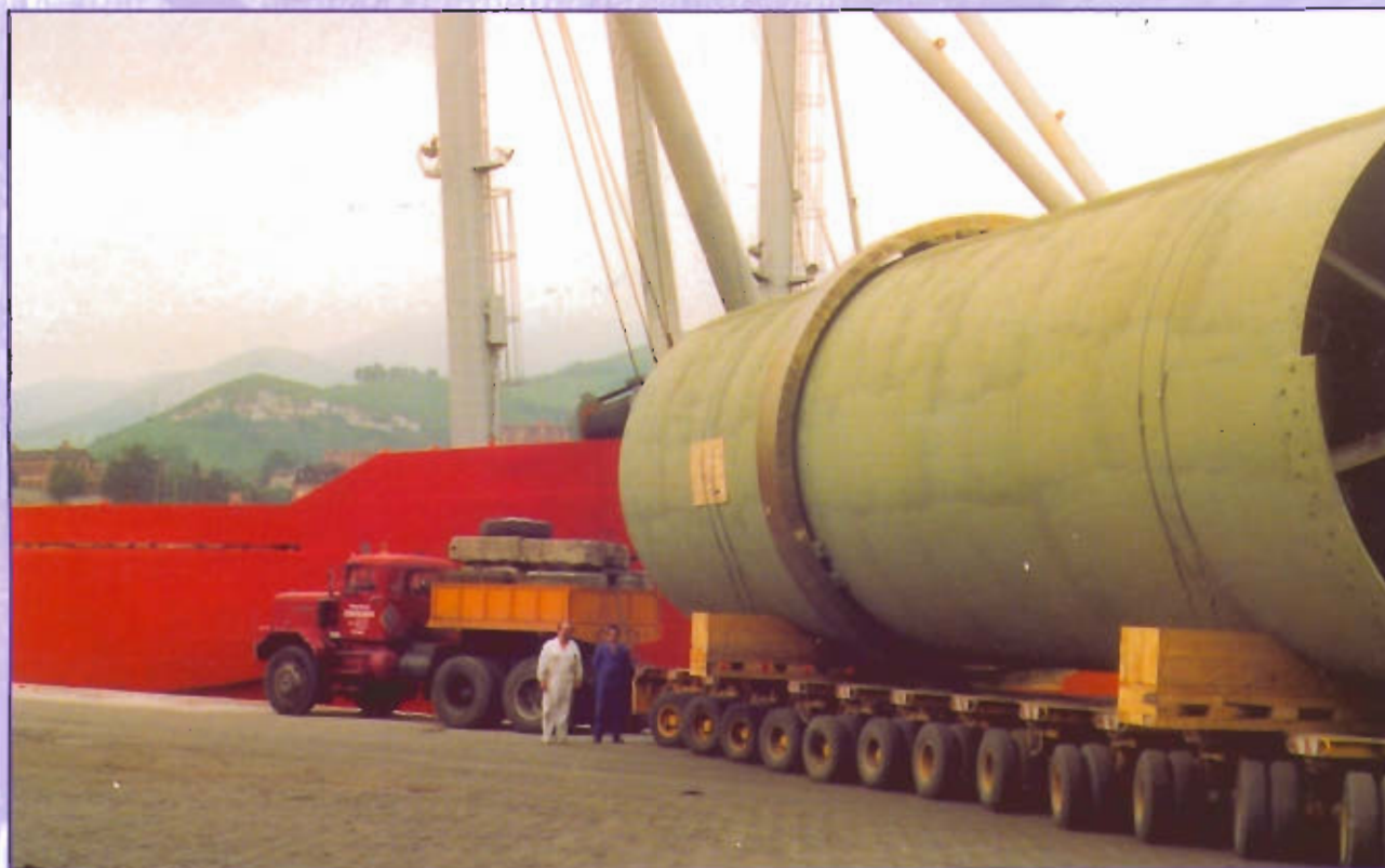
Rotary Dryer Ø 4,95 m. x 31,5 m. L for NPK, DAP and GTSP • SABIC-TPL (SAUDI ARABIA)
