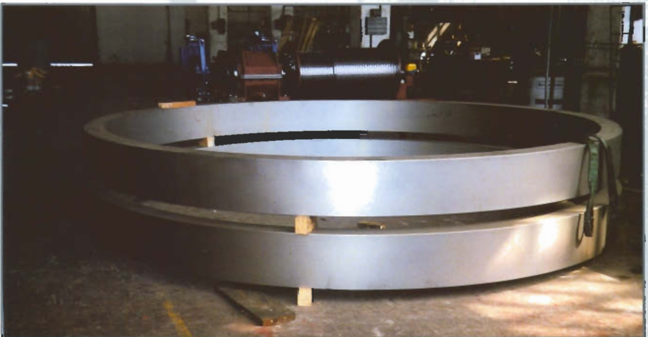
Riding ring. Installation of Pequiven-VENEZUELA
