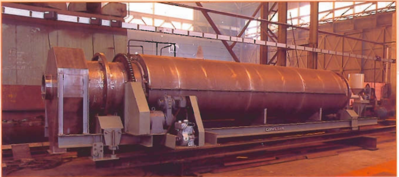
Dehumidifier drum for barks. MECAPEÑA-BILBAO-SPAIN
