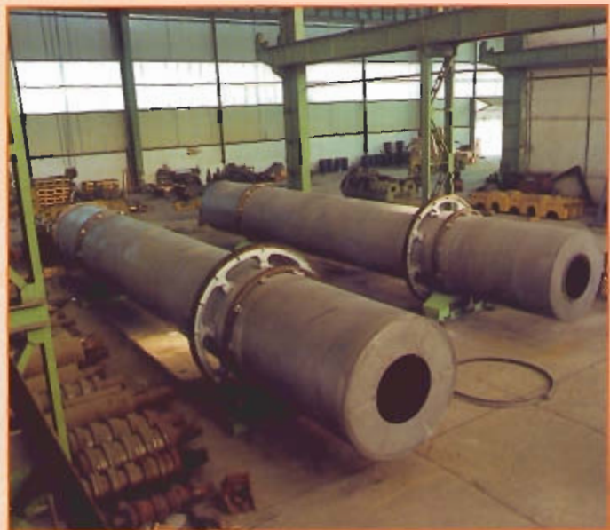
Cooler and Dryer Drums in stainless steel of ammonium sulphate PHILPHOS - PHILIPPINES
