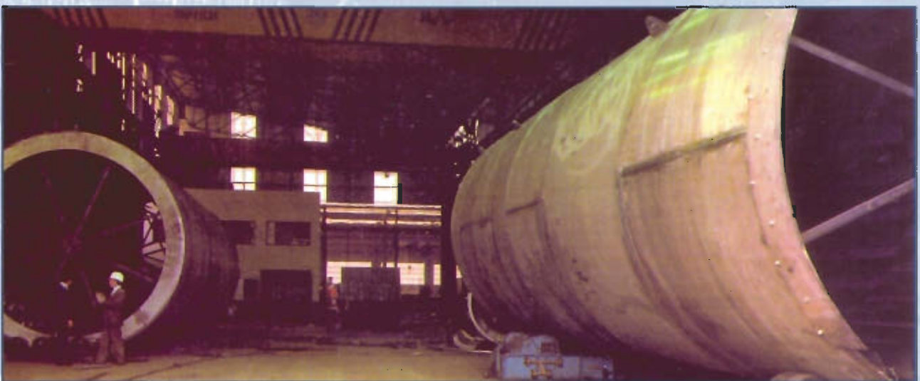
Rotary drum in solid stainless steel for ammonium nitrate, thickness 50 mm. Dimensions Ø 4,5 m x 30 m L FERTIBERIA (SAGUNTO-SPAIN)
