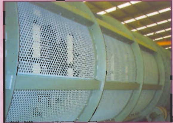
Classifier Trommel for Waste Material PLACOSOL-URBASER MALAGA-SPAIN
