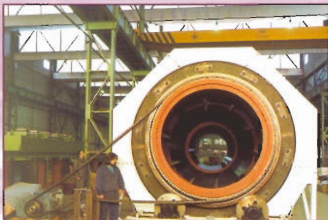
Crusher Ø 3,5 m x 9,1m L for coal GUAVIO-COLOMBIA
