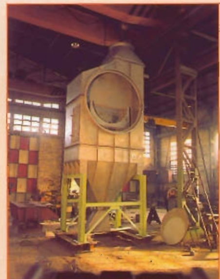
Transfer box in stainless steel for Cooler and Dryer Drums
