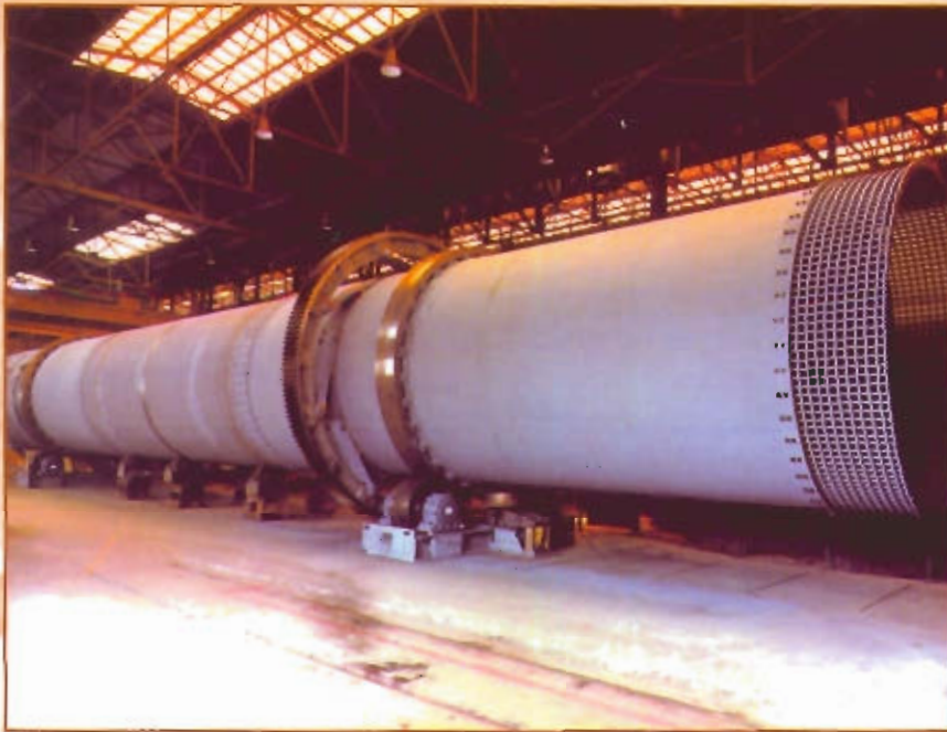
Rotary Dryer for Granulated Fertilizers Ø 3,2 m x 28 m L INABONOS ROULLIER GROUP (LODOSA-SPAIN)
