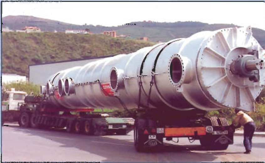
Indirect Dryer of PVC Ø 3,2 m x 28 m L. Group ACETEX (CANADA)
