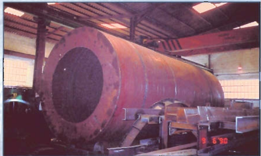
Granulator of NPK for Petroquimia GRESIK II (INDONESIA)
