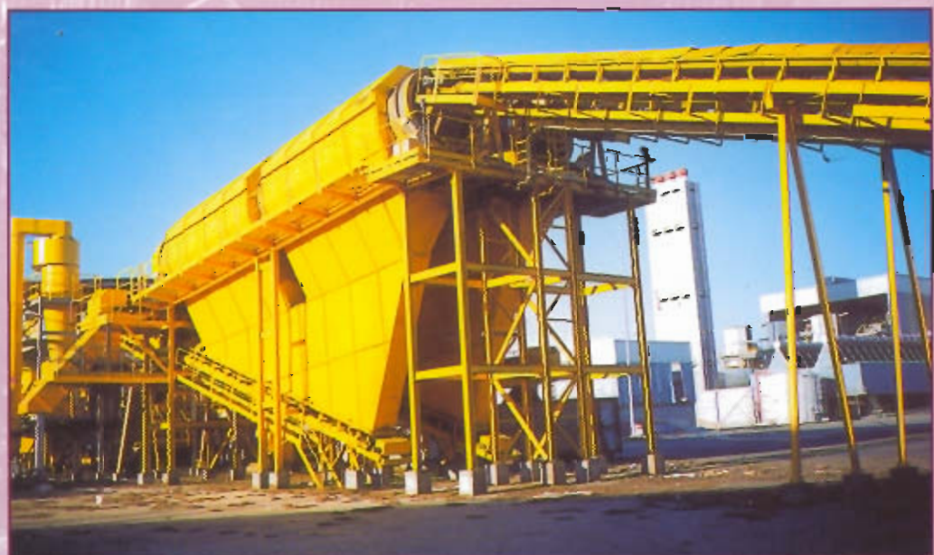
Classifier trommel for Waste material DRAGADOS-TIRIADRID- SPAIN
