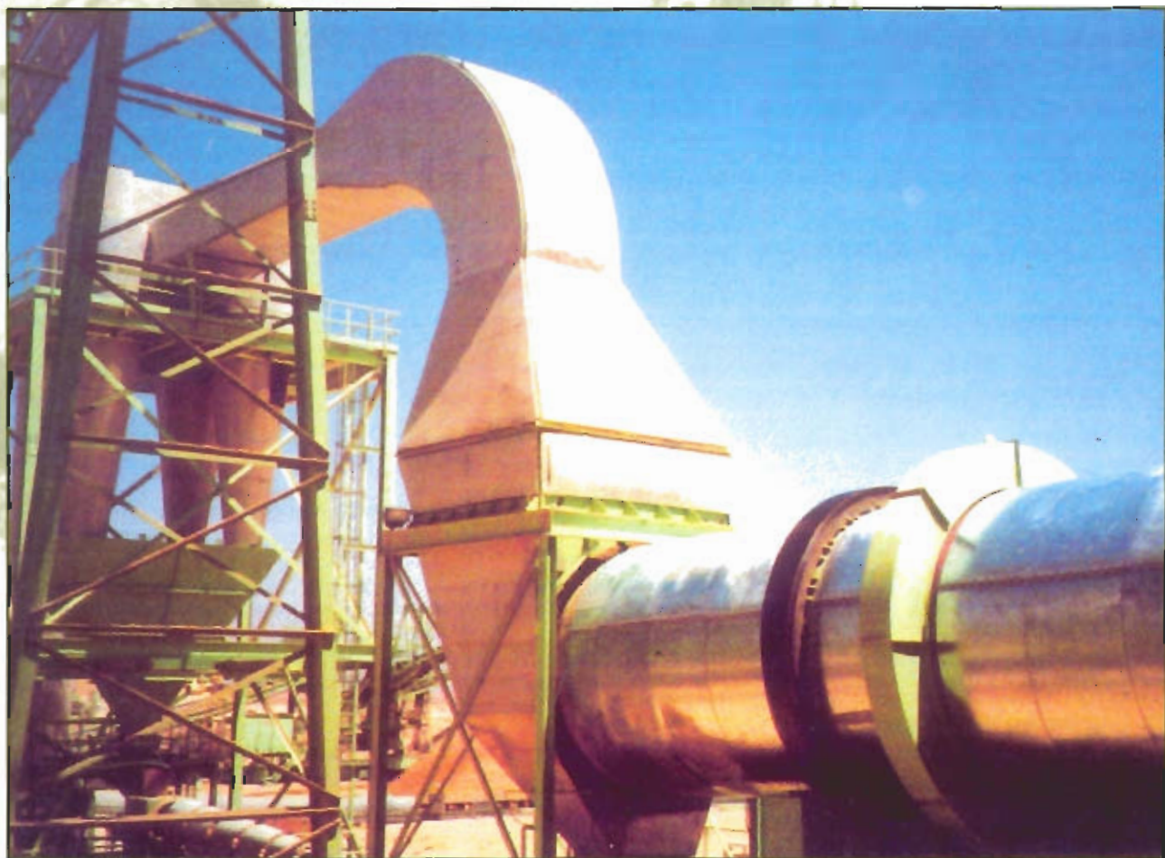
Calcinator for flyight ashes Ø 2,8 m L x 22 m L. INDUMETAL-BILBAO-SPAIN
