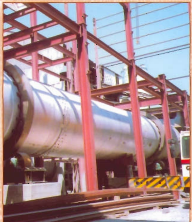
Rotary Dryer for NPK Ø 3 m x 24 m L CNCCC-GUIXI-CHINA
