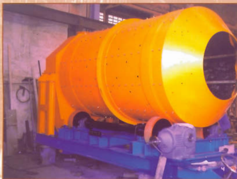
Granulator Drum for Bicalcic Phosphate TIMAC-SAINT MALO- FRANCE
