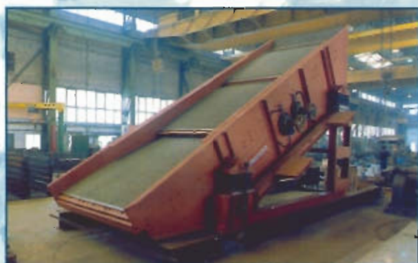
CRIBLE INCLINÉ 2500 x 8000 mm DOUBLE ACT. MECANIQUE LUZHAY - CHINE
