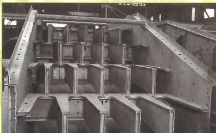
Prescreener Feeder Extractor type 2000 x 6000 mm. Capacity 1800 T/h (Phosphate 0-1500 mm). Separation 200 mm OCP MOROCCO
