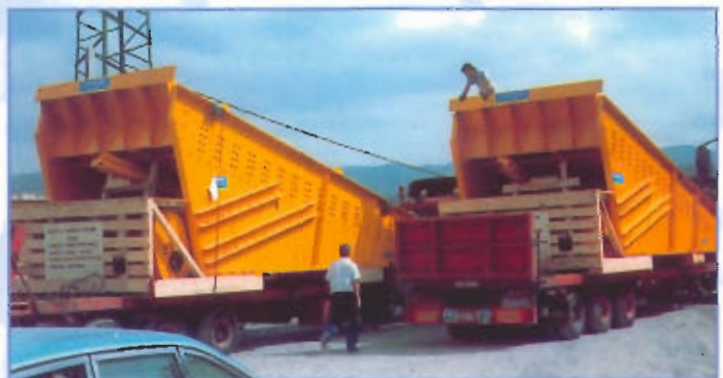
Feeders Type 2750 x 8000 mm. Capacity 3800 T/h Guavio - COLOMBIA
