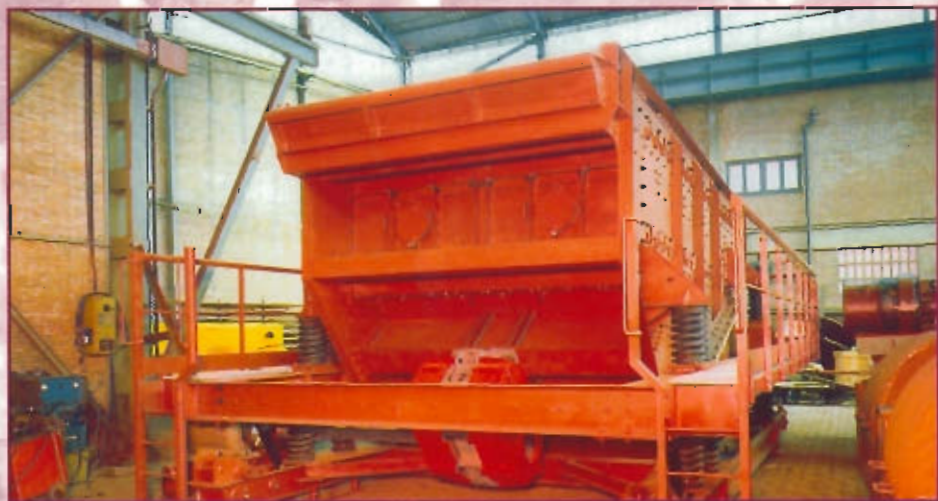
Horizontal Screen with counterweight. Iron mineral Capacity: 600 T/h. Type 2000 x 7000 mm Hispanobras (BRAZIL)
