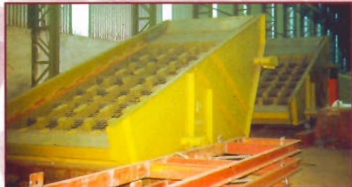
Cleaning Screen. Coal. Capacity: 2500 T/h. Type 2000 x 7000 mm Endesa - SPAIN
