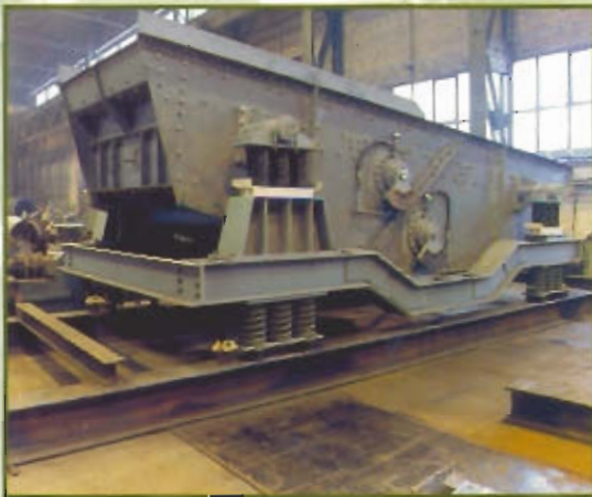
Exciters mounted on counter-weight Capacity 80 T/h. Type 2200 x 7000 mm Organic waste . Barcelone (SPAIN)
