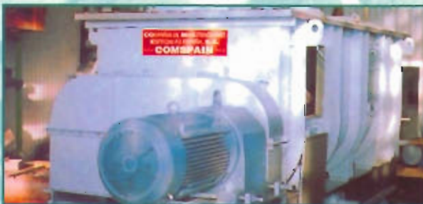
Mixer for 100 T/h smelted urea-mixture, etc NPK-DAP plant. DONGBU CHEMICAL - KOREA
