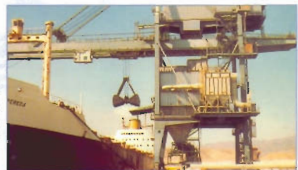
Distributors Unload boats with exciter Type 2800 x 3000mm Capacity: 2500 T/h KRÜPP Germany to ALMERIA - SPAIN
