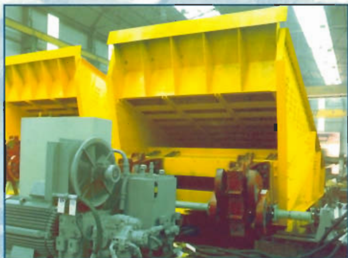
FEEDERS 3000 x 8000 mm Capacity: 5000 T/h. Grain-size 0-2000 mm - AUXINAM - ECUADOR
