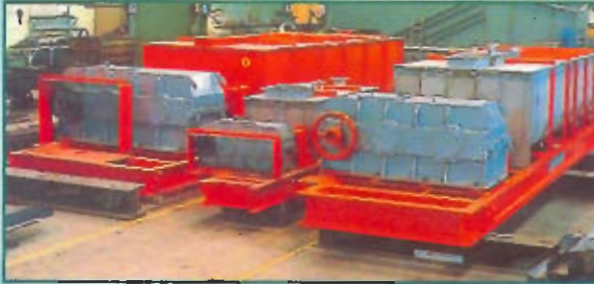
Double screw granulators for 240 T/h of NPK ZORKA AZOTARA SUBÓTICA NPK, NA - YUGOSLAVIE
