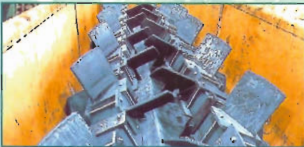
NPK 300 T/h granulator dismountable type of paddles NOVOMOSKÓWSK - RUSSIE
