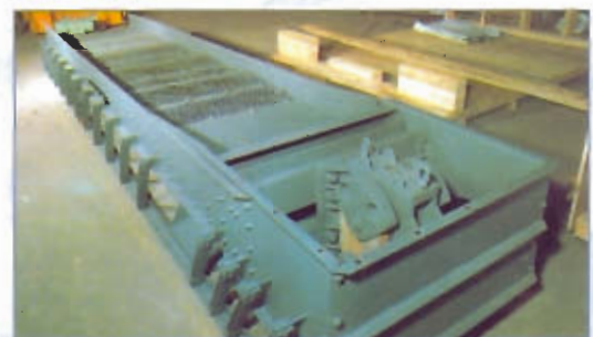
Cooler Distributor Type: 800 x 2000 mm Coke. Capacity: 40 T/h - NIGERIA
