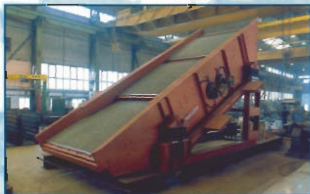
INCLINED SCREEN 2500 x 8000 mm DOUBLE MECHANICAL DRIVE LUZHAI-CHINA
