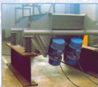
Extractor with motovibrator. Type 800x1500mm Capacity: 120 T/h PEQUIVEN - VENEZUELA
