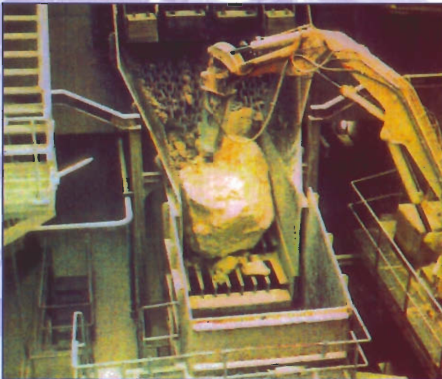
Prescreener Feeder. Type 2500 x 10.000 mm Capacity 1500 T/h (size 0-1300 mm) Detail of Crushing Hammer SOLVAY - FRANCE
