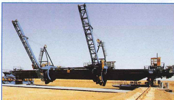
Reclaimer type bridge with two bucket wheels of 3,500 t/h: ENDESA (As Pontes de Garcia Rodríguez, Spain) Coal, KOCH technology.
