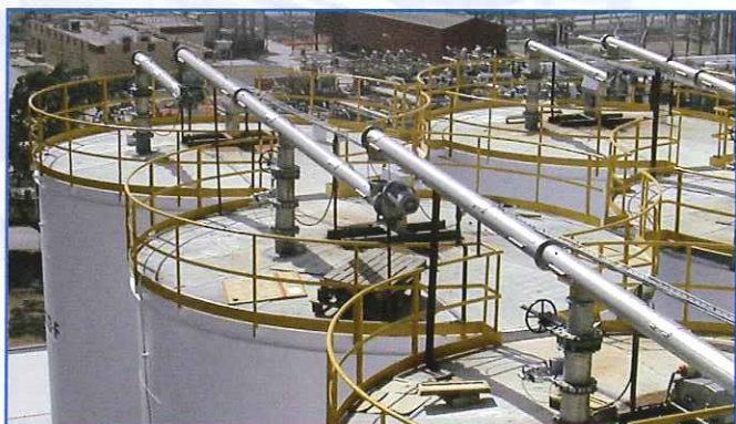
Screw conveyors and silos: FOSFATOS DE CARTAGENA (Escombreras, Spain) Monocalcium Phosphate and Dicalcium Phosphate.
