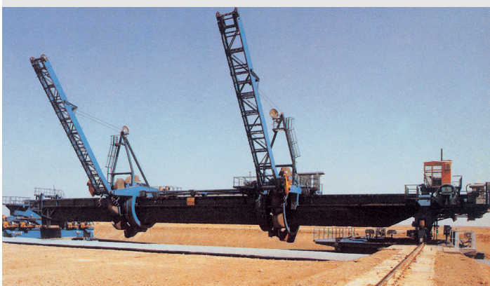
Reclaimer with two bucket wheels of 3,500 T/h: ENDESA (As Pontes de García Rodríguez, Spain) Coal, KOCH technology.
