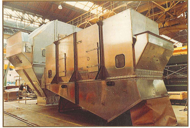
Static Fluid Bed for Ammonium Sulphate.
