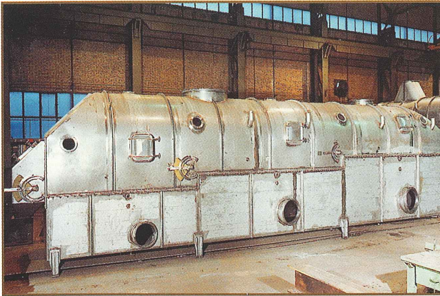
Static Fluid Bed «cascade» for reactions-drying-cooling.
