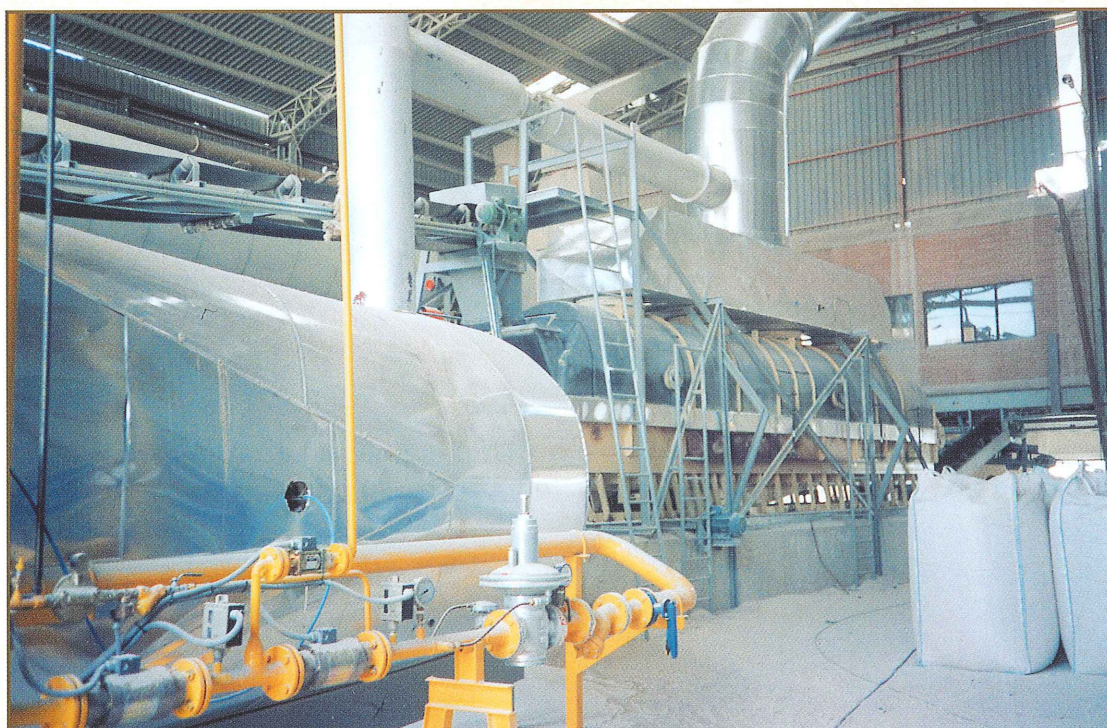
Drying Vibrating Fluid Bed (High temperature) for sepiolite-clays (400° C).
