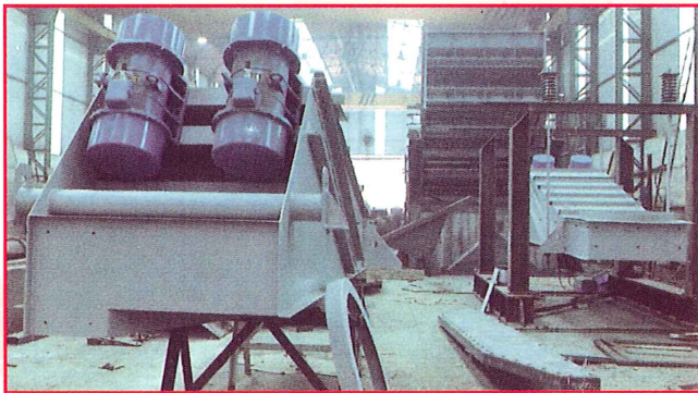
2 vibrating feeders, NPK, 1,500 x 3,500 mm, 190,000 kg/h. National Fertilizer Co. (Taiwan).
