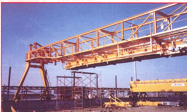
Stacker and reclaimer for Compost, composting plant. Dragados (Spain).
