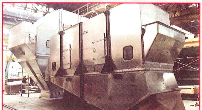
2 fluid bed coolers, NP, 2 x 34 m 2 , 150,000 kg/h. Toyo Engineering (China).
