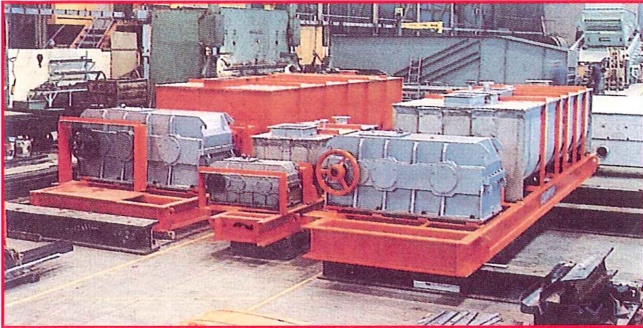
Double screw granulators for 240 T/h of NPK. Zorka Azotara Subótica NPK, NA. (Yugoslavia).
