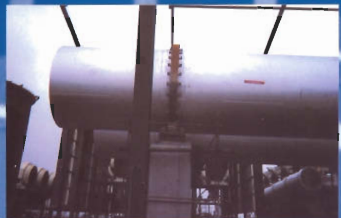
Drying drums. 3,6 m diameter x 25 m Length.
