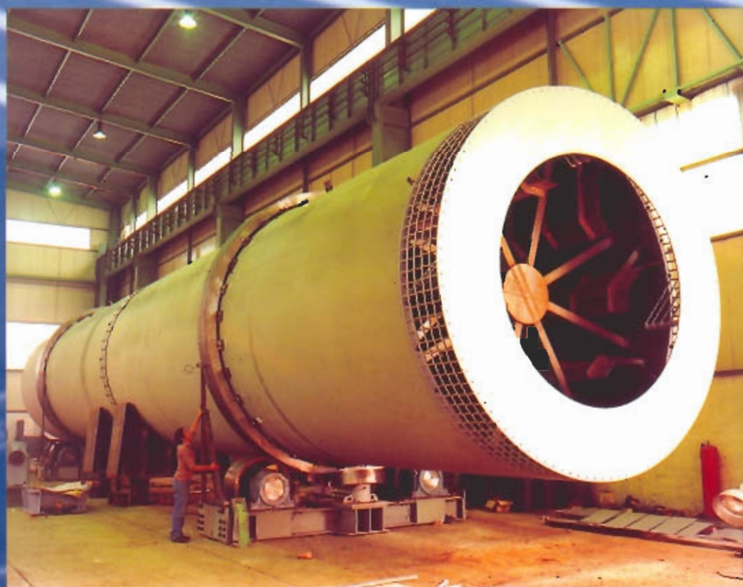
Drying drum. 4,6 m. of diameter x 29 m. length.
