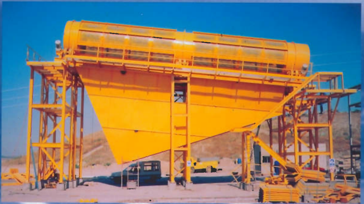
Refining trommel for compost.
