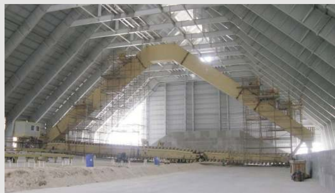
Portal scraper at the indoor storage park for phosphate and additives of 21,300 m 2 and 160,000 T for the whole chemical complex of Ras Az Zawr. Customer: MA'ADEN/WORLEY PARSONS – Engineering: LITWIN.
