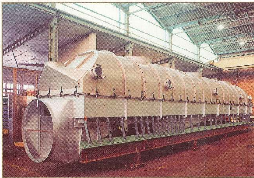
Vibrating Fluid bed supported by blades.
