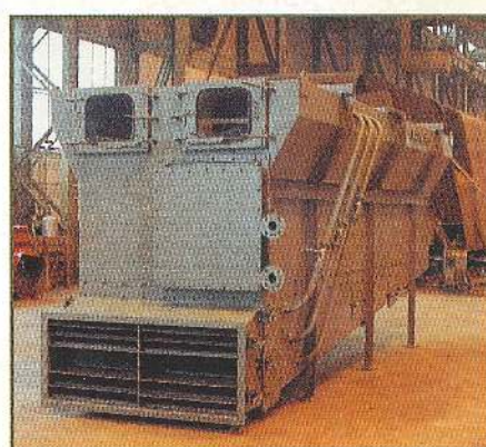
Fluid Bed with exchanger for sodium sulphate.
