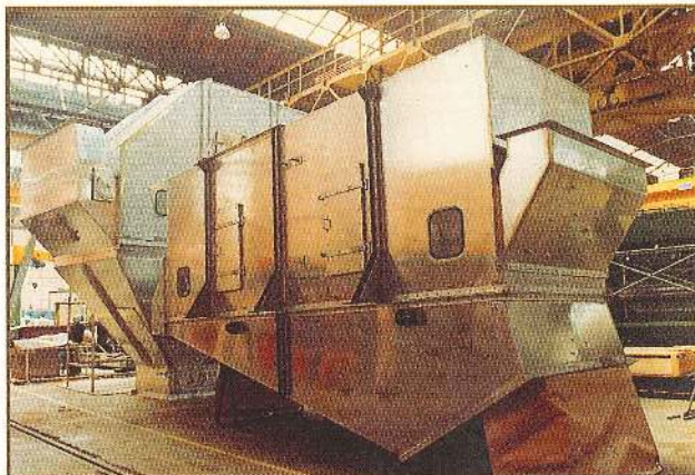
Static Fluid Bed for Ammonium Sulphate.
