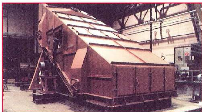
2 processing screens, NPK, 2,000 x 5,000 mm, 200,000 kg/h. Namhae (Korea).
