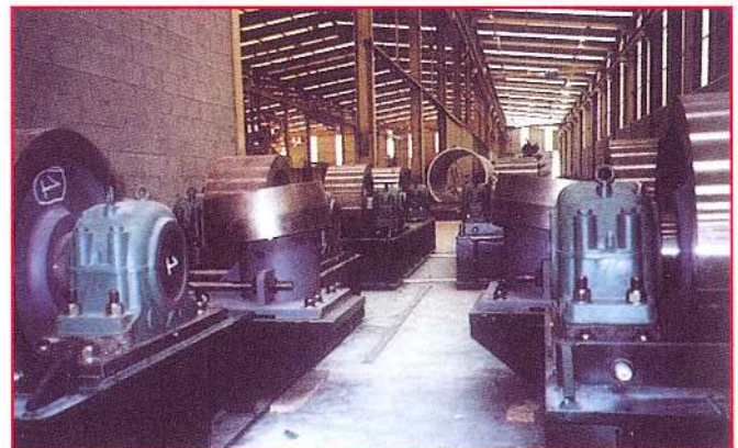
Rolling system for a NPK plant, 310,000 T/h. Petrokimia (Indonesia)
