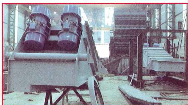
2 vibrating feeders, NPK, 1,500 x 3,500 mm, 190,000 kg/h. National Fertilizer Co. (Taiwan).
