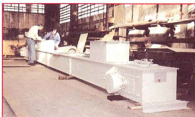
Chain conveyor for 250 T/h, GTSP, General Fertilizet Co. Homs (Syria).
