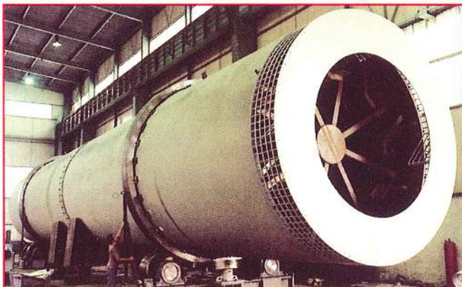
Dryer rotary drum, NPK-DAP, \varnothing 4.6 x 30 m, 360,000 kg/h. Siape/Gabes (Tunisia).
