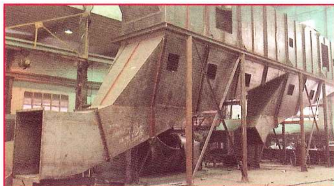
Cooling fluid bed, AN, 32 m 2 , 75,000 kg/h. Fertimex (Mexico).
